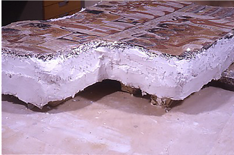
Fig. 11 Nebamun paintings: the separation layer Paraloid B72 and glass micro balloon paste, used between the arriccio and the foaming epoxy resin (image with courtesy of the Trustees of the British Museum)
