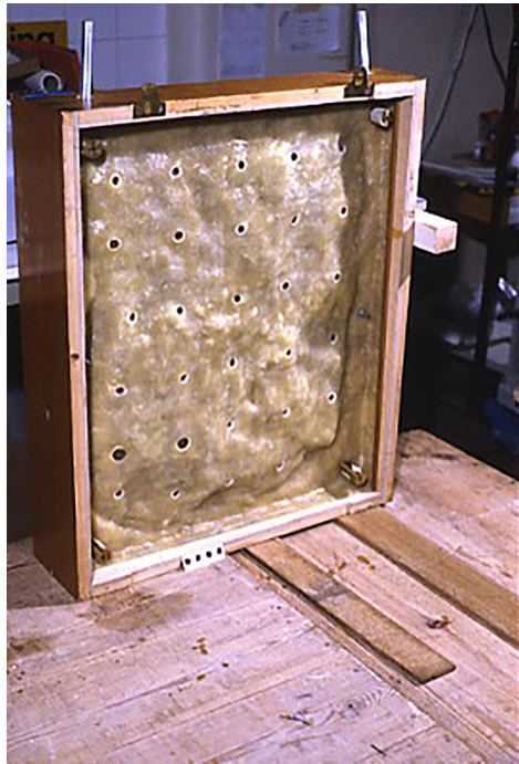
Fig. 12 The removable polyester resin and glass fibre backing plate from the 1982 mounting of Banquest (guests and musicians) (image with courtesy of the Trustees of the British Museum)
